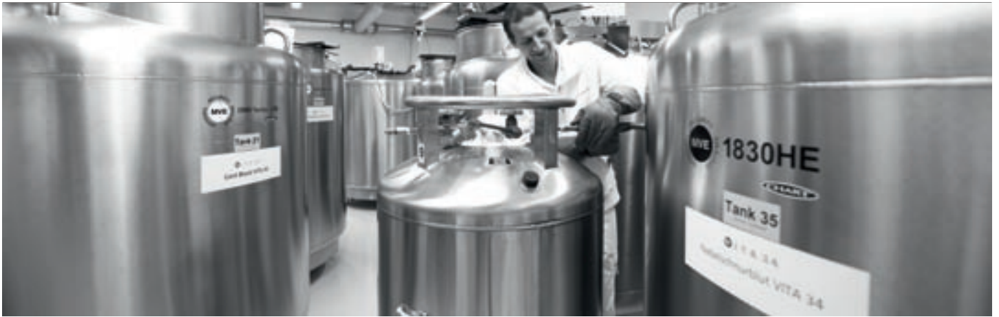
Filling a storage tank with nitrogen
